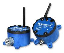
**Wzzard Wireless Mesh** Sensing Nodes are tailor-made for bringing hard-toreach sensor data into SCADA and IIoT solutions. Wzzard sensor nodes are battery powered and IP67- and C1D2rated, making them easy to integrate even in harsh environments. They utilize Smartmesh IP, a self-forming, self-healing wireless mesh protocol that not only provides a highly-reliable and resilient network, but is also easy to deploy.
