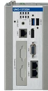
The UNO-1372GH is designed to be safely operated in hazardous locations and are UL listed for Hazardous Locations with Class I, Division 2, groups A, B, C, D T4A certification.
